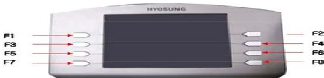
- Function Key Location on ATM -
