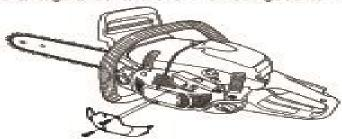
CAUTION! If the special winterising kit has been fitted or any measures, have been taken to increase the temperature these changes must be reversed before the machine is used in normal temperature conditions. Otherwise there is a risk of overheating, resulting in severe clamage to the engine.
