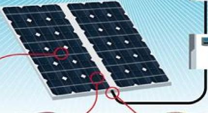
Photons hit the solar panel, knocking electrons free of the silicon atoms within the solar cells.
