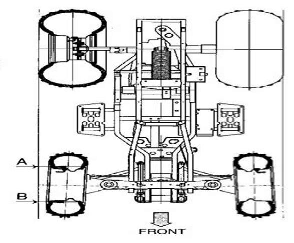
NOTE: The steering post arm (freg) can be used as an indicator of whether the handlebars are straight. The freg should always point straight back from the steering post when handlebars are straight.
