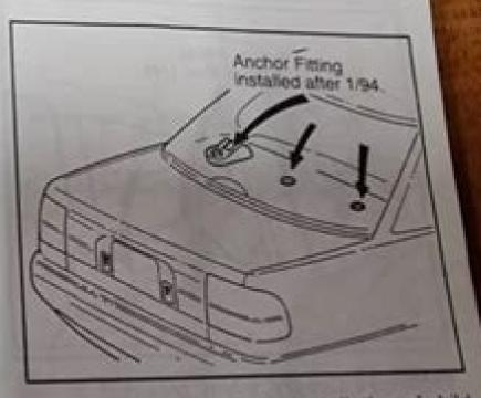
Anchorage points for the installation of child restraint anchor fittings are provided in the locations shown in the above and following illustrations.
