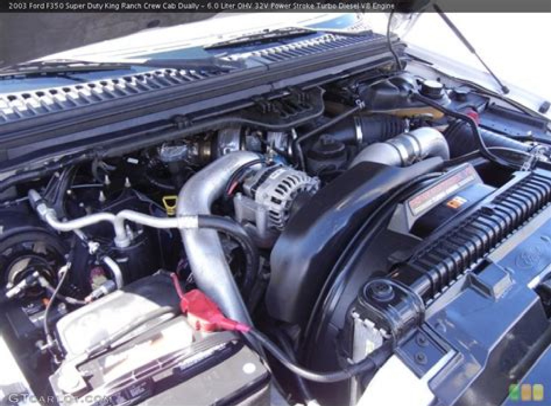
2003 Ford F350 Super Duty King Ranch Crew Cab Dualy - 6.0 Liter OHV 32V Power Stroke Turbo Diesel V8 Engine
