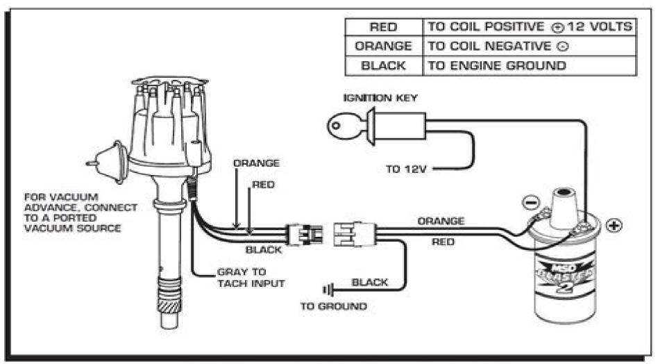
Figure 10 Wiring the Ready-to-Run Chevrolet Distributor.
