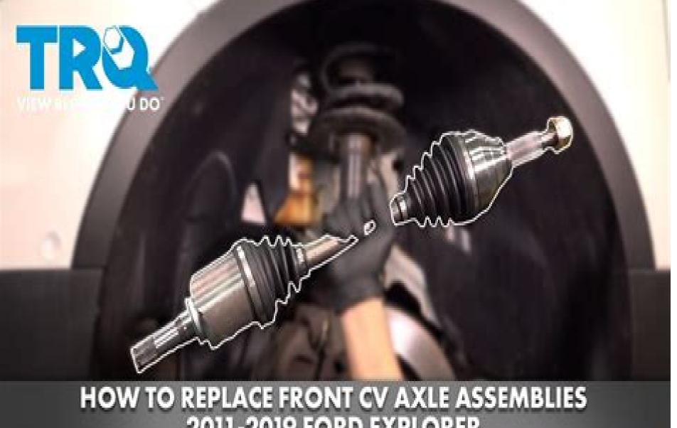
HOW TO REPLACE FRONT CV AXLE ASSEMBLIES 2011-2019 FORD EXPLORER
