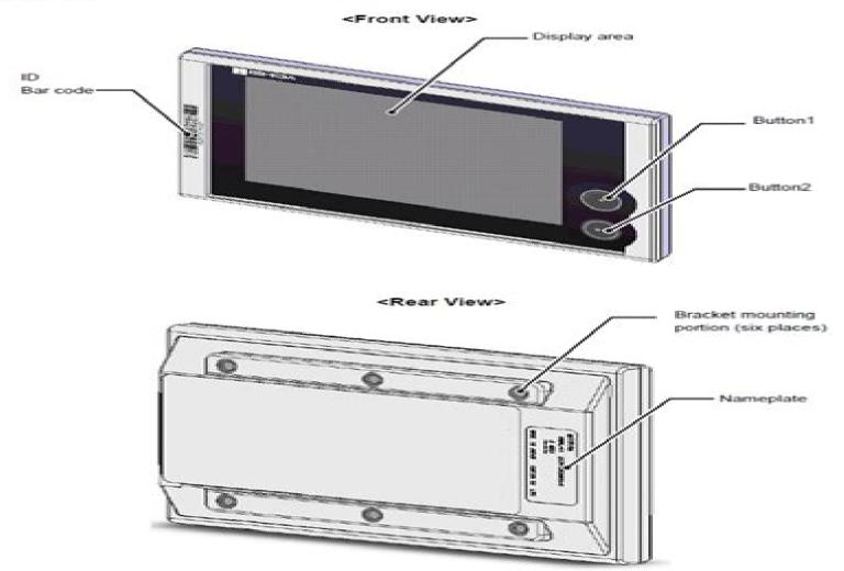
Power ON ← OFF: Hold down [Button1] and [Button2] simultaneously.
