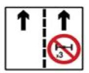
In a tunnel goods vehicles cannot use right-hand lane (by reference to number of axles)
