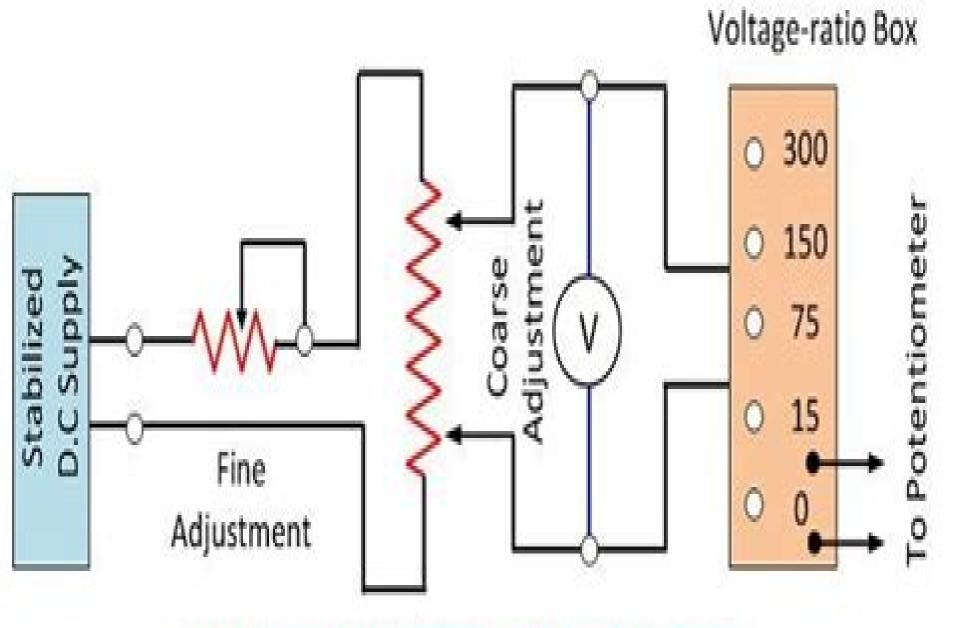
Calibration of Voltmeter with Potentiometer
