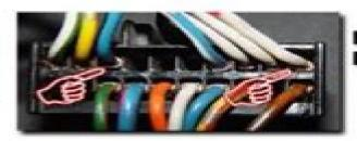
B5 = VTEC Pressure Switch B19 = Knock Sensor
