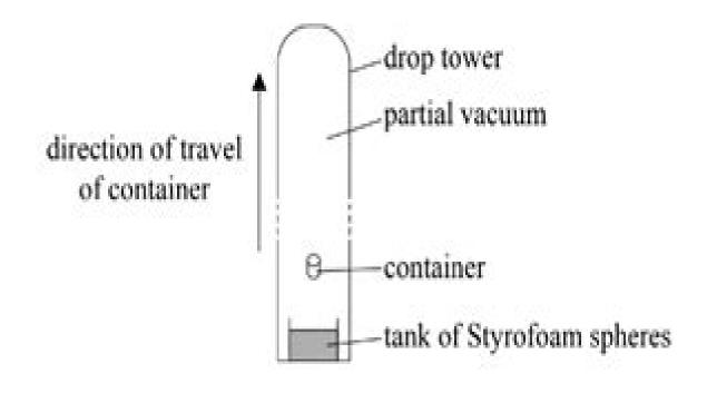
The container moves under the influence of gravity and eventually falls back to the bottom of the tower. Most of the air is removed from the tower so that air resistance is negligible. While in flight, the container and its contents are in free-fall.
