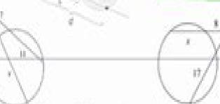
Secants & Tangents Theorem: If a secant segment and tangent segment are drawn to a circle from the same external point, the product of the length of the secant segment and its external part pare of the length of the tangent segment. Formula:  $a \cdot b = c^2$
