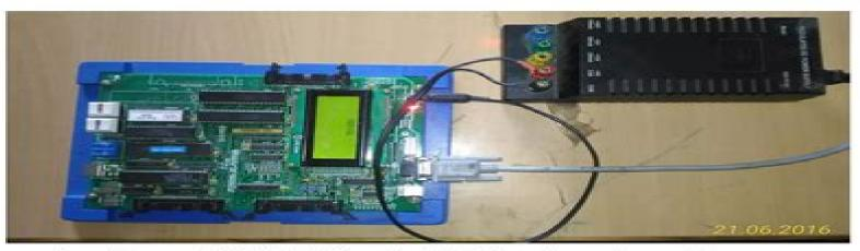
We connect the ESA cable from the 8051 MC to system male connector.
