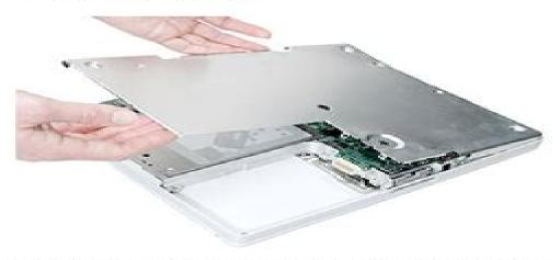
5. Note: The two springs in the battery compartment can become loose. When reassembling the computer, make sure that the two springs are in place before installing the bottom case. Each spring has grease on the coils, and each has a plastic cap on one end. Make sure the cap fits securely on the spring, and the curved side of the cap is positioned against the inner frame.
