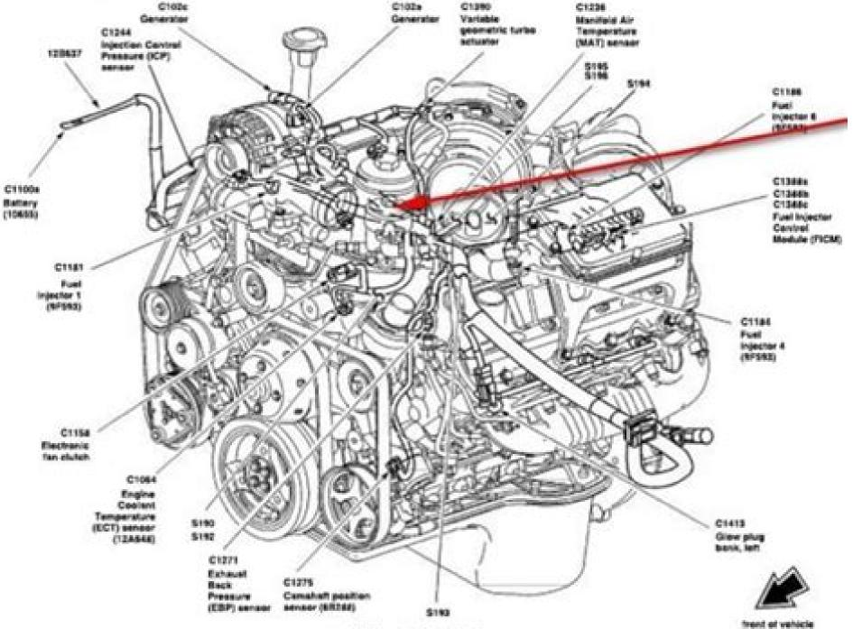
6.CL Diesel engine, LH side
