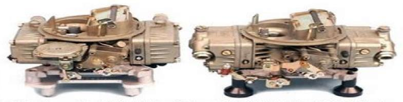
This side-by-side comparison of fuel-bowl styles makes them easy to identify. At the left is a 4160 (PN 1850) carb equipped with a side-hung float. At the right is a 4150 carb with a center-hung float. The 4150 carb has a metering block at the secondary side; the 4160 has a secondary metering plate. A 4160 is easily converted to the 4150 configuration.
