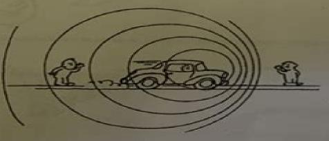
When an automobile moves toward a listener, the sound of its horn seems relatively
