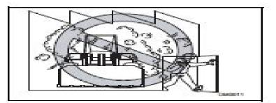
Do not start to work in an enclosed area if adequate ventilation is not provided. Furnes could build up during operation that could cause drowsiness, injury, or death.
