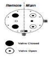
Main Tank is in Service and Remote Tank is in Brine Rinse.
