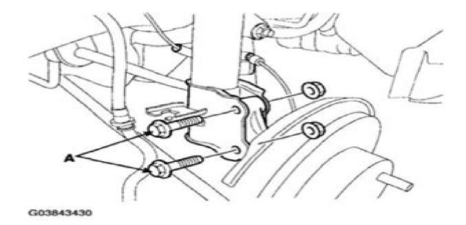
Fig. 7: Removing Lower Strut Mounting Bolts Courtesy of HYUNDAI MOTOR CO.
