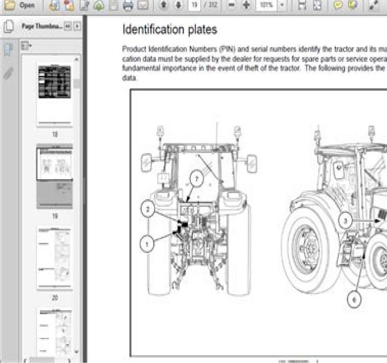
Product Identification Numbers (PIN) and serial numbers identify the tractor and its main components. The identification data must be supplied by the dealer for requests for spare parts or service operations. Identification data is of fundamental importance in the event of theft of the tractor. The following provides the locations of the identification
