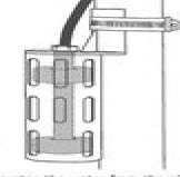
second switch. As the pump evacuates the water from the pit, the floats will deep. The pump will run for an additional 10 seconds to extend the cycle after the float returns to its original position.
