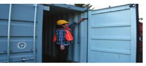
Attach the CSD at the right doorframe. It will stay in place with the use of built-in magnets.
