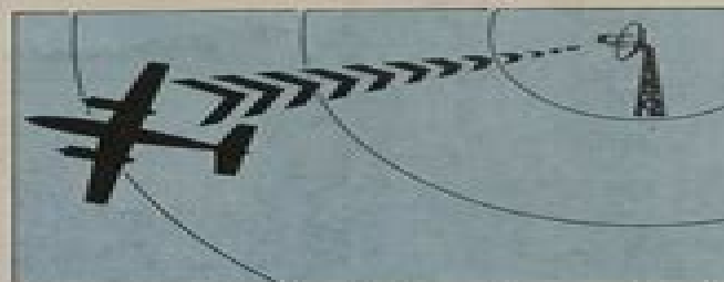
Transponder-pulsed transmitter replies to radar station.
