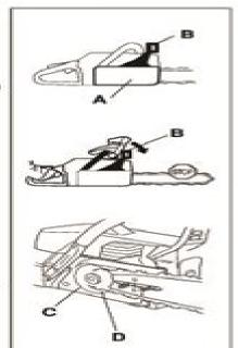
2 The front hand guard is not designed solely to activate the chain brake. Another important safety feature is that it prevents the chain from hitting your left hand if you lose your grip on the front handle.
