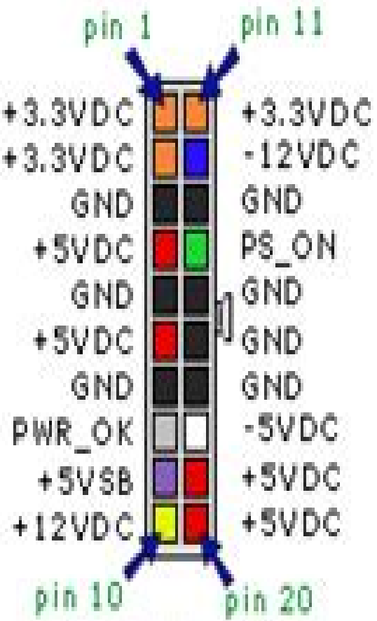
ATX 20 pin Molex Main Power Connector
