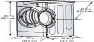
\* Most installations require a minimum 5 1/2 in. (14 cm) clearance behind the dryer for the exhaust vent with elbow.
