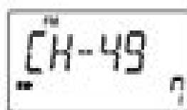
Channel indication mode example (Memory ch 49 of memory bank 7)
