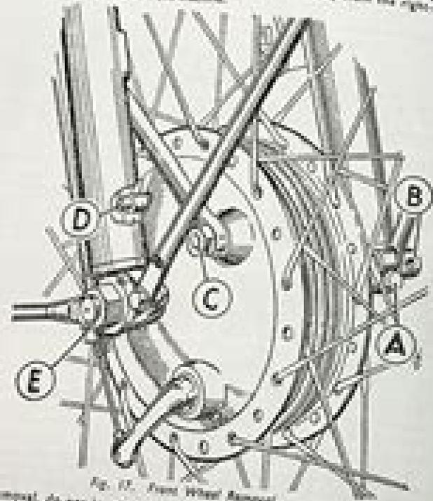
Fig. 17. Front Wheel Removal.
