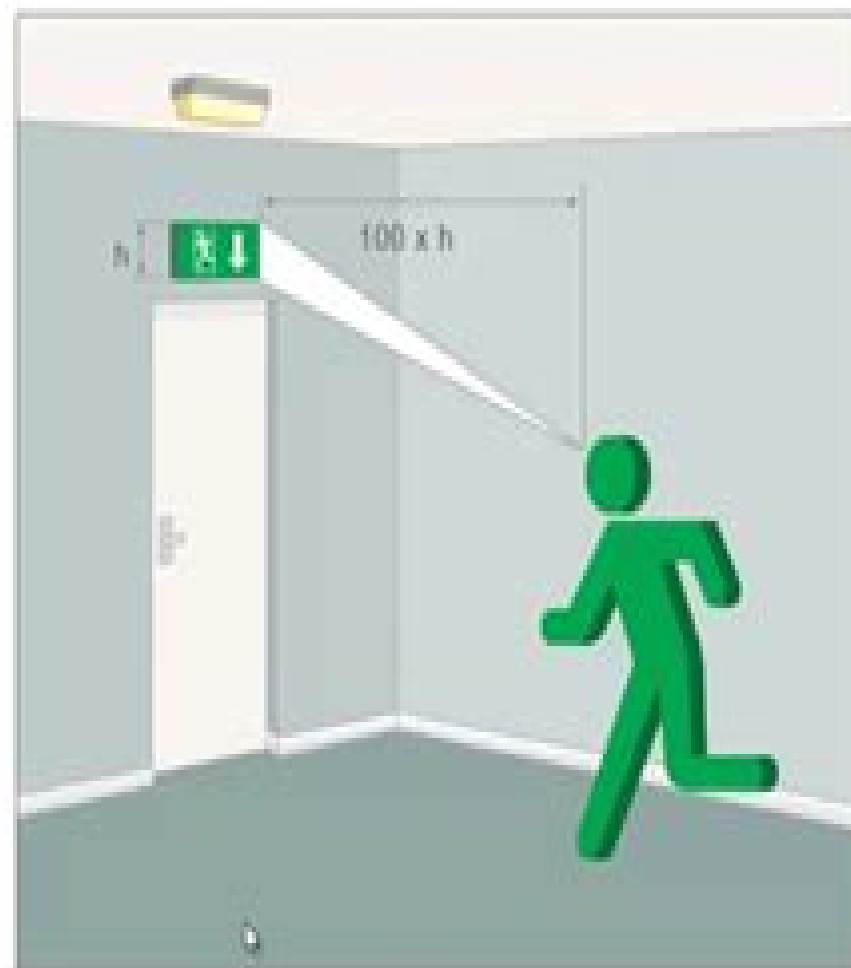
Externally illuminated signs - 100 \times the panel height
