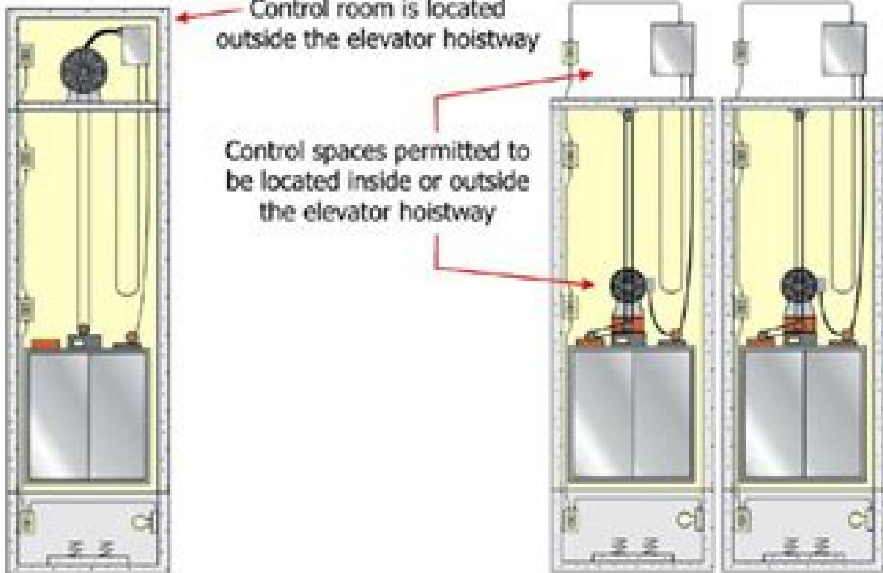
Article 620 defines spaces as well as rooms for elevator motor controller
