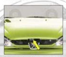
From outside: lift the catch and open the bonnet. Secure the strut to hold the bonnet open.
