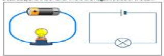
This picture shows time cell landed up to a light bulb. Niptice the ottoget lines in the timout diagram, represent rows. The cell is one long line and a short one (this is not a lightery line tre still call it one!)
