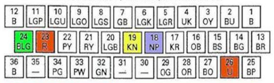
Crankshaft position sensor pin 23 = sensor pin 26 = ground
