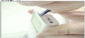
Using the included flathead screwdriver, CAREFULLY pry off the white plastic top of the iPod Mini. It may help to note that SLIGHTLY squeezing the sides of the device can create more space between the white plastic piece and the metal case. It also helps to press toward the metal case rather than the plastic. The white top may be attached with glue.
