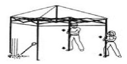
For height adjustments pull ring on leg and slide the frame up to desired height. Release ring to lock the pin into the hole on the leg.
