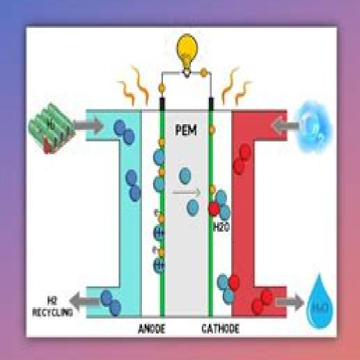
How HYDROGEN FUEL CELL Works?
