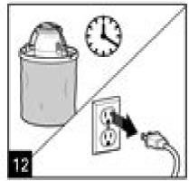
ice cream will churn for about 20 to 40 minutes depending on the recipe. Ice cream is ready when the motor stops or slows down. Unplug from outlet to turn off motor.
