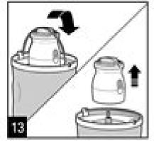
To remove the canister, push down on the locking button, move unit so that the power cord on the motor is on the opposite side or away from you, and move the handle toward you. Remove motor.
