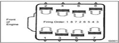
The cylinder numbering for each engine is as shown in diagrams.
