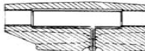
Axle pivot (Cast iron I-Beam axle)
