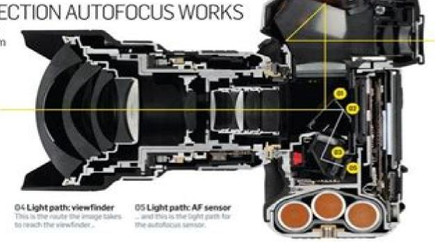
Unlike most other types of digital camera, digital SLRs use separate 'phase-detection' AF sensors
