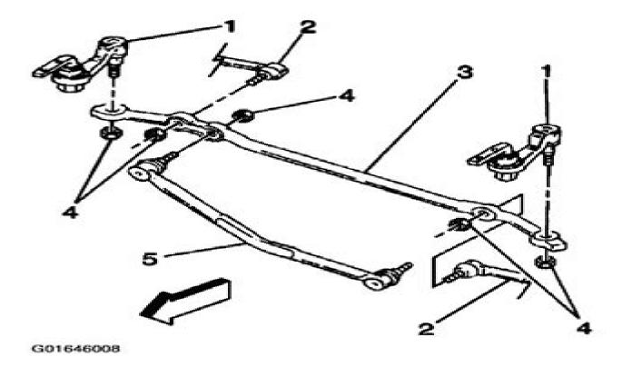
Fig. 41: Installing Prevailing Torque Nut To Idler Arm Ball Studs Courtesy of GENERAL MOTORS CORP.
