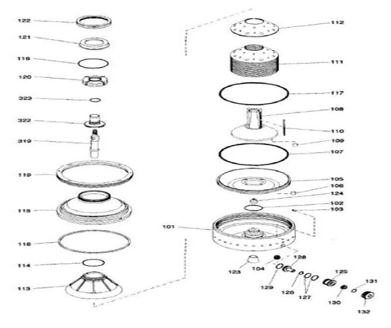
Fig. 2-31 Bowl Assembly Drawing (SJ10F, 15F, 30F)
