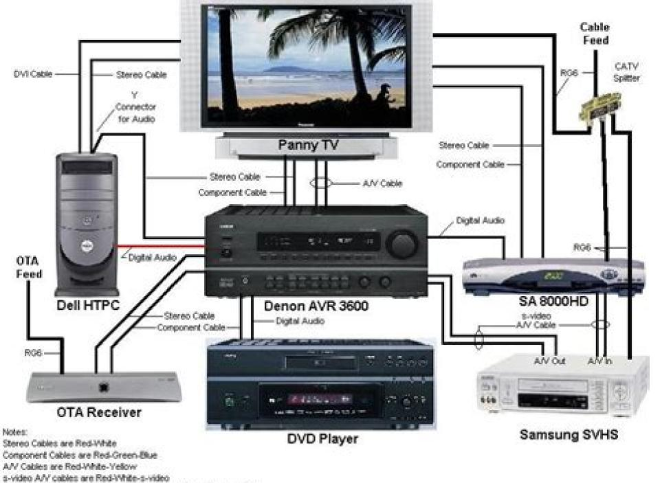
Diotal Audio Cables are as required by the equipment connections
