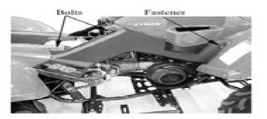
Remove the two bolts, fastener and left side cover.
