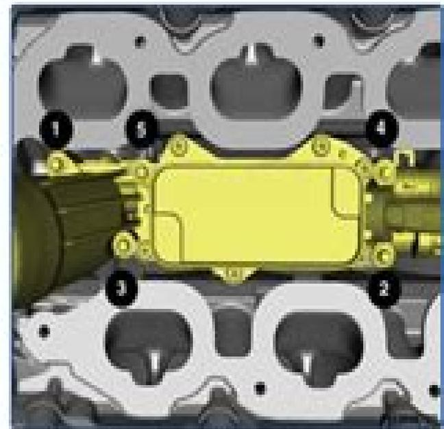
5. Install the heater hose (1) to the oil filter housing
