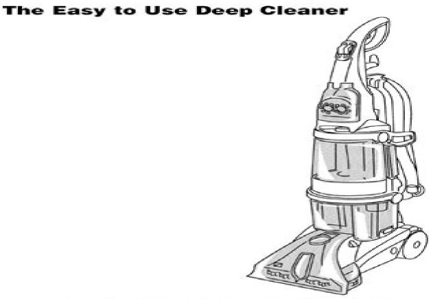
SteamVac™ V2™ Deep Cleaner cleans carpet fibers by applying hot tap water and cleaning solution.
