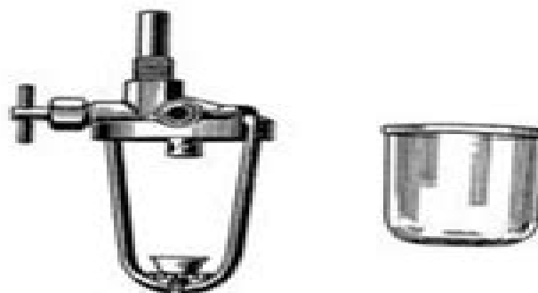
Illustration No. 10 Fuel strainer showing glass bowl removed for cleaning.
